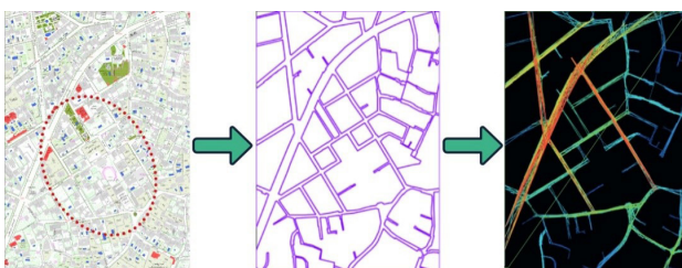
Fig. 4. Converting the city map into a map of convex spaces and then forming an axial map. Source: Author.
