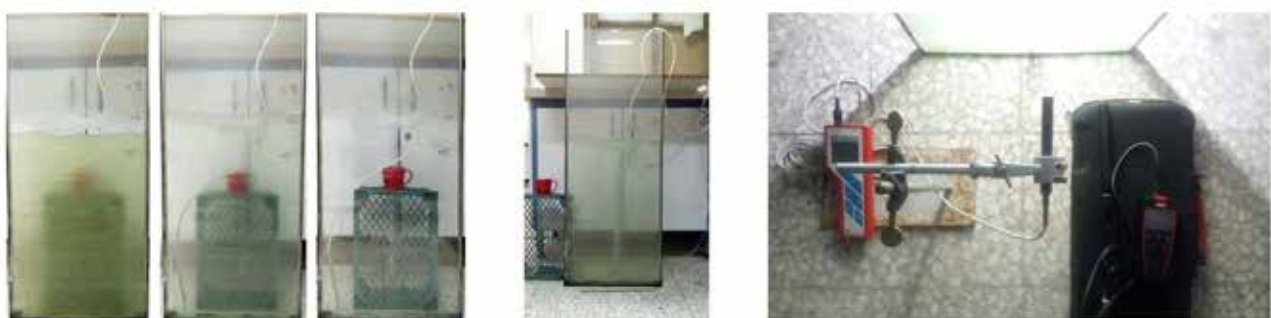
Fig. 3. the manufactured bioreactor and the equipment used in the testing process. Source: Authors.
