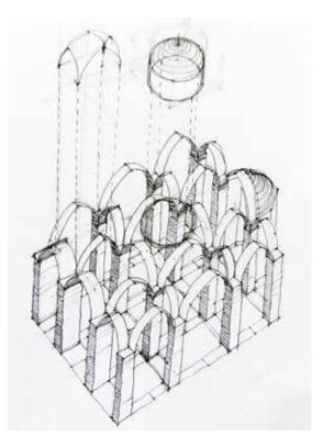
Fig.8. the structure of dome and vaultsof St. Stephen Church. Source: authors.
