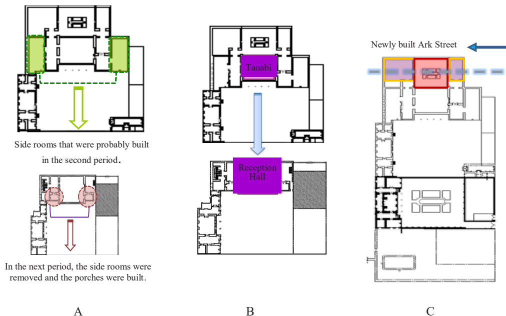
Fig. 8. An overall view of house's changes on the northern side. A: Changing the earrings to the balcony , B: Converting Tanabi to the hall & C: Destroying the inner part with the construction of a new street. Source: Authors.
