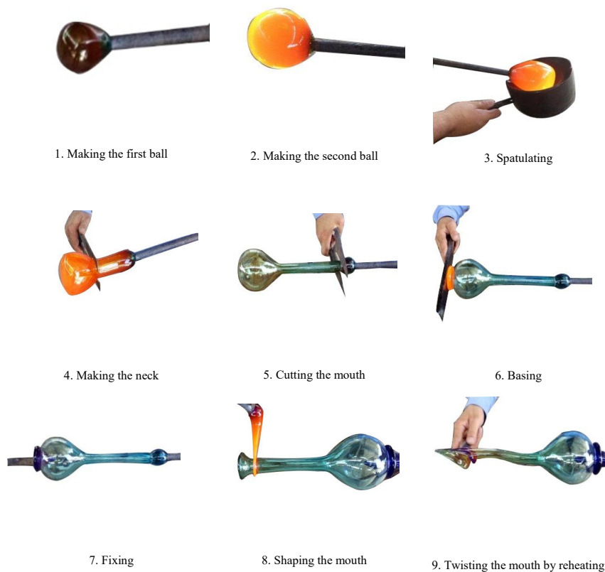
Fig.2. Different stages of making carafes and Ashkdans in Alvan Bolour glass factory. Source: Authors.
