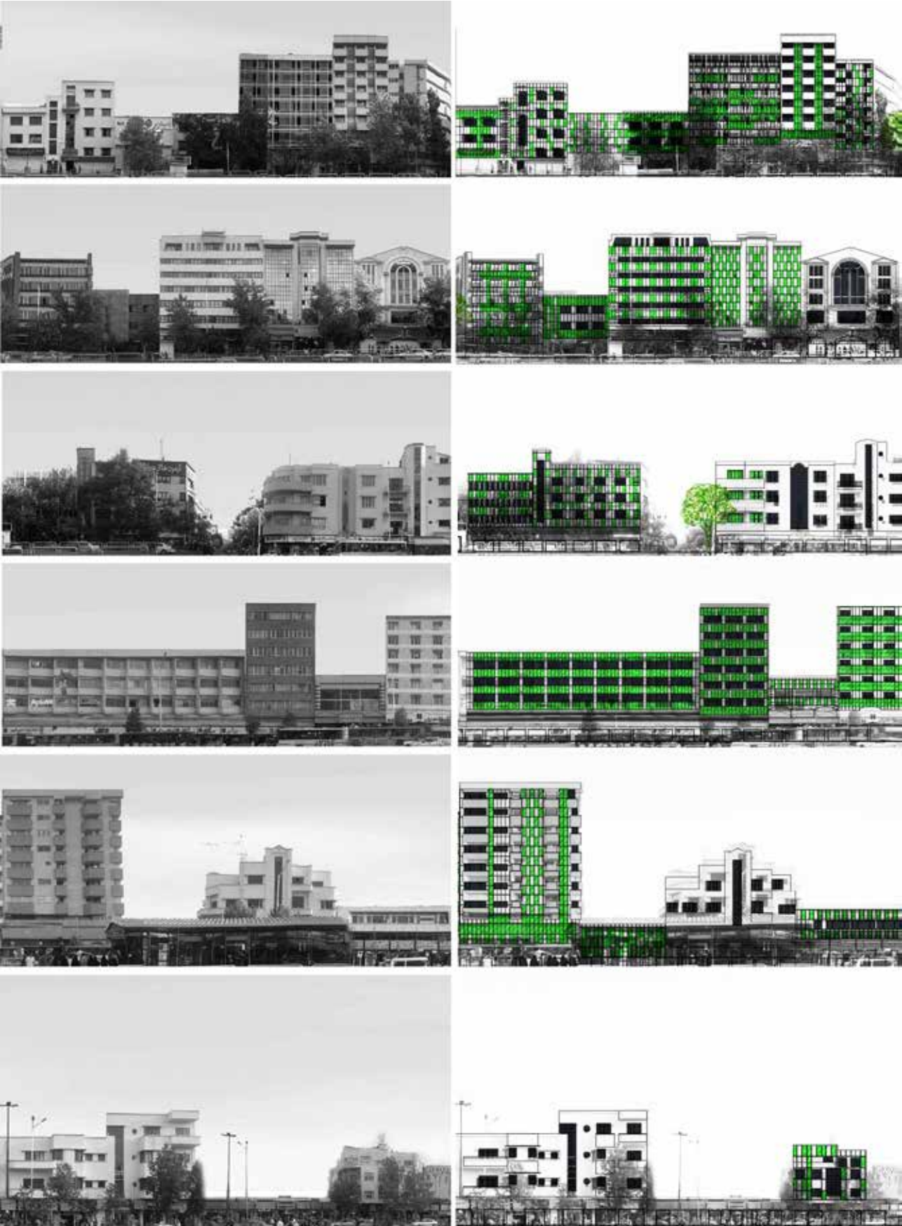
Fig. 1-b. Comparing the south façade of Enghelab Street with and without microalgae panels. Source: Authors.
