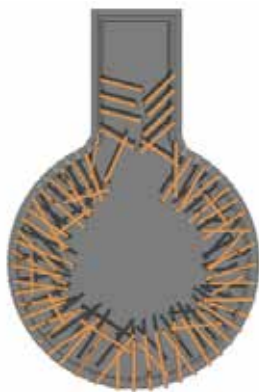
Fig. 4. A matrix of wooden mesh applied into the GST. The details of this wooden mesh are observed by means of endoscopic technique used by the authors, 2017. Photo and modeling by A. Moradi.
