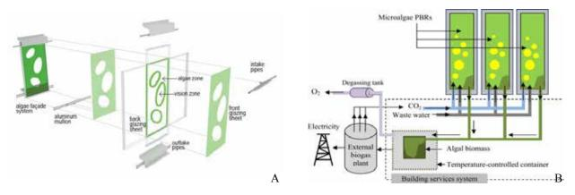
Fig. 5. A) demonstration of an algae façade's components. B) Operation mechanism of algae façade. Source: Elrayies, 2018.
