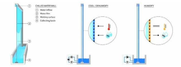
Fig.3. A representation of a watery wall details. Source: Fraunhofer Institute, 2018.
