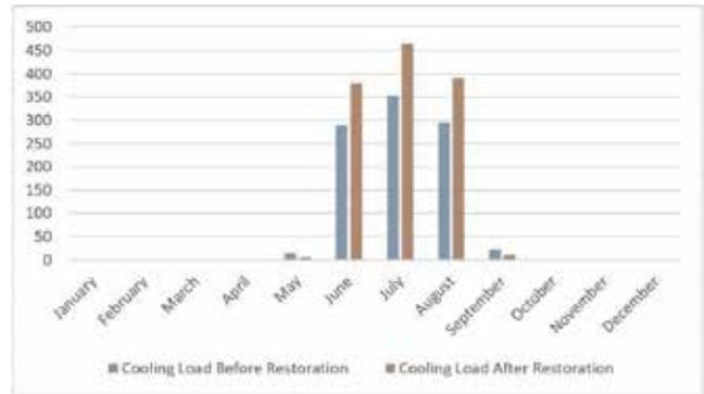
Diagram 5. Cooling load of Dodari room in Oloomi’s house before and after restoration. Source: authors.
