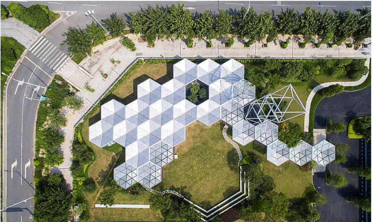
Fig. 10. Open architecture and development of a six-sided rebuilding construction system by the modularity strategy in Guangzhou, China. Source: Pirbabaei & Amraei, 2009.
