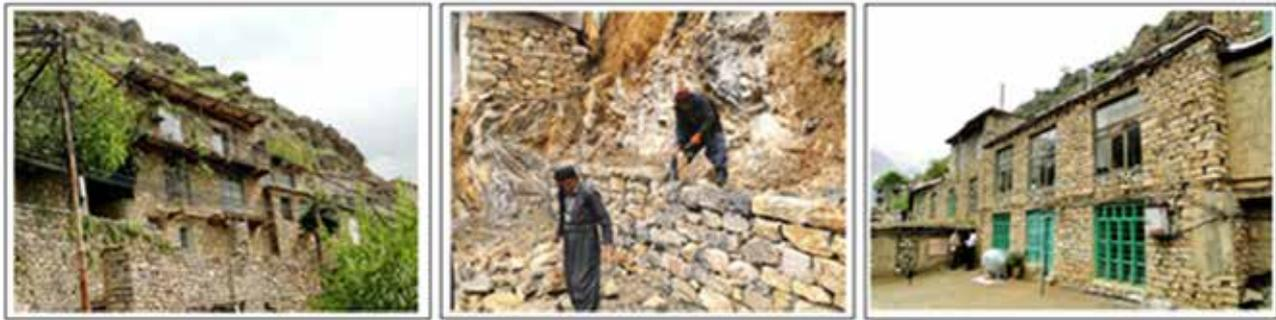
Fig. 4. Stone, wood and soil are the main materials of construction on Hawraman. Source: authors.
